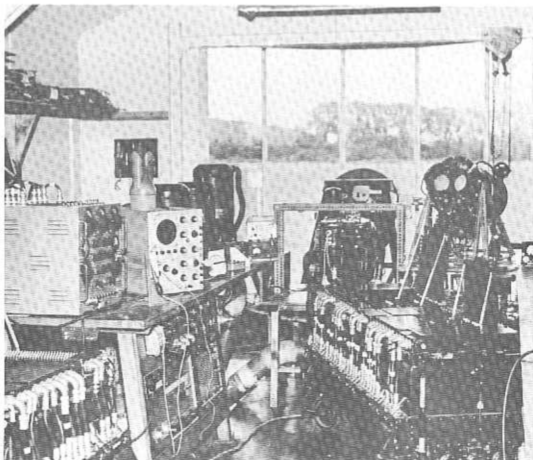
Radar test bay laid out to test the airborne radar as a system, also main and ancillary equipment for checking overall performance, and Servo loop responses.
