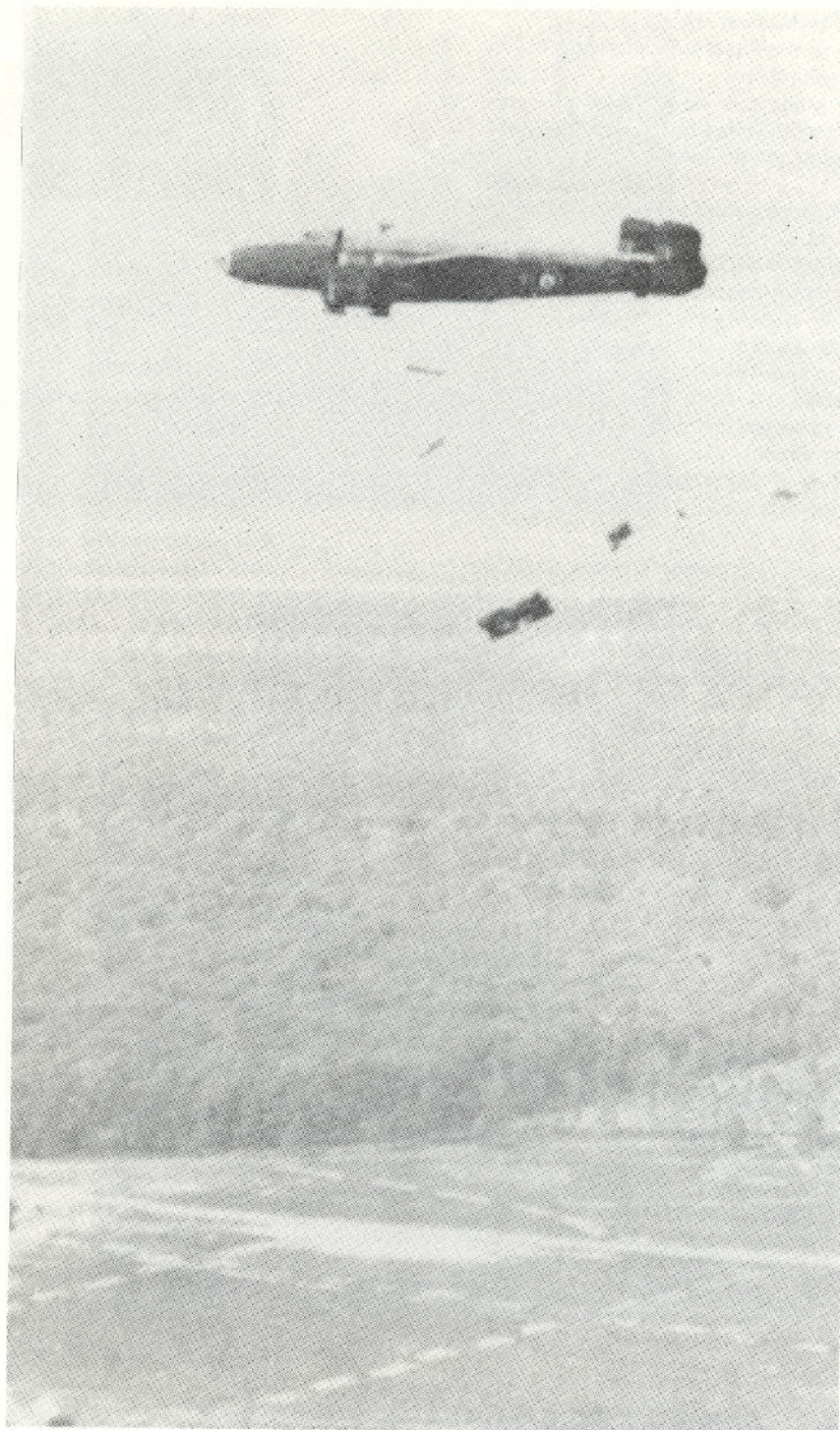
Fig. 117. A jeep & supply containers drop from a Halifax during trials at Beaulieu.
